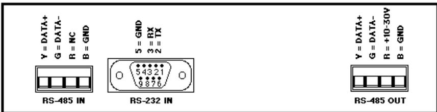
Figure 1B Connections for SCM9B-A2000.
