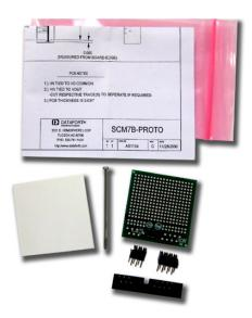
Figure 2: SCM7B-PROTO Breadboard Kit.
