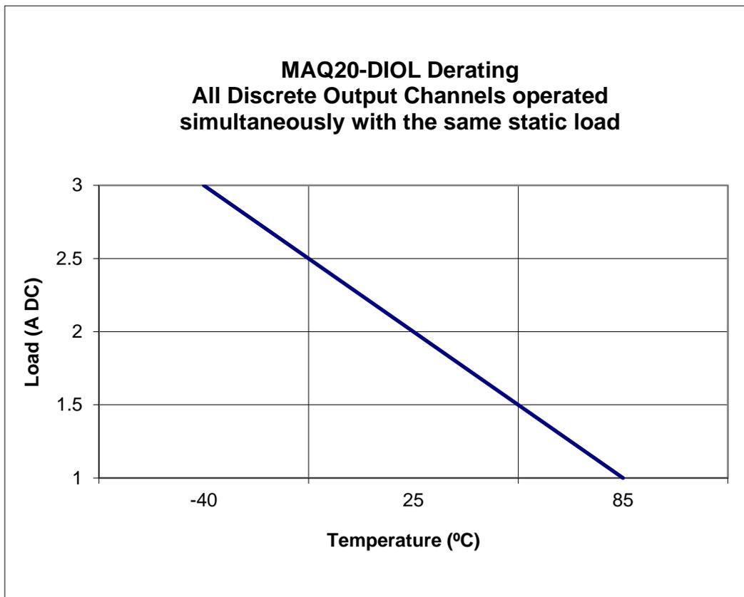
Figure 16: MAQ20-DIOL Derating for Static Loads
