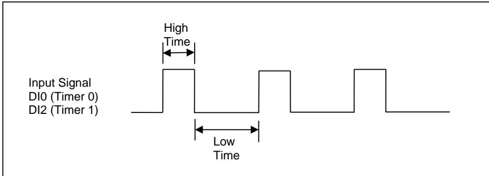
**Figure 10: Waveform Measurement Parameters**
