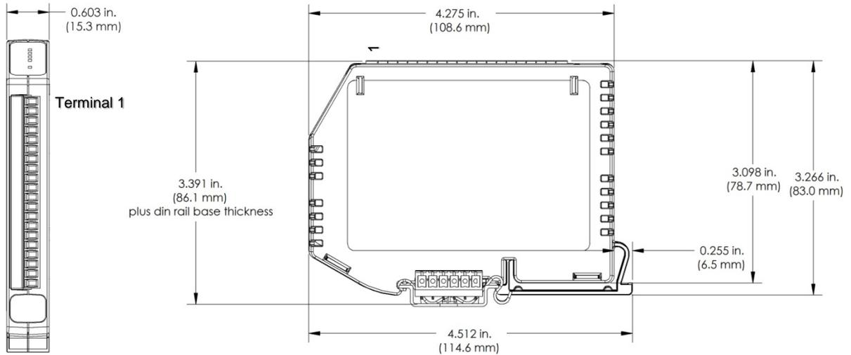
Figure 1: Module Dimensions
