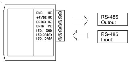
Figure 1 Connections for SCM9B-D192.
