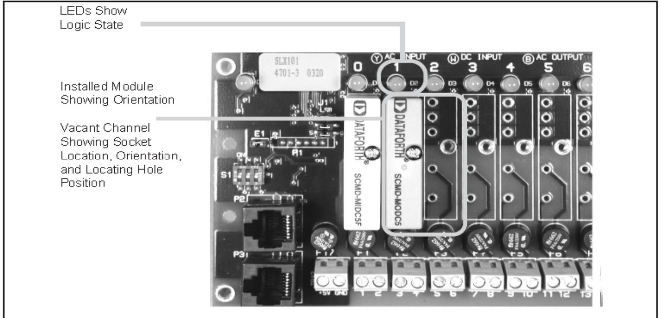
Figure 2: SCMD Module Installation
