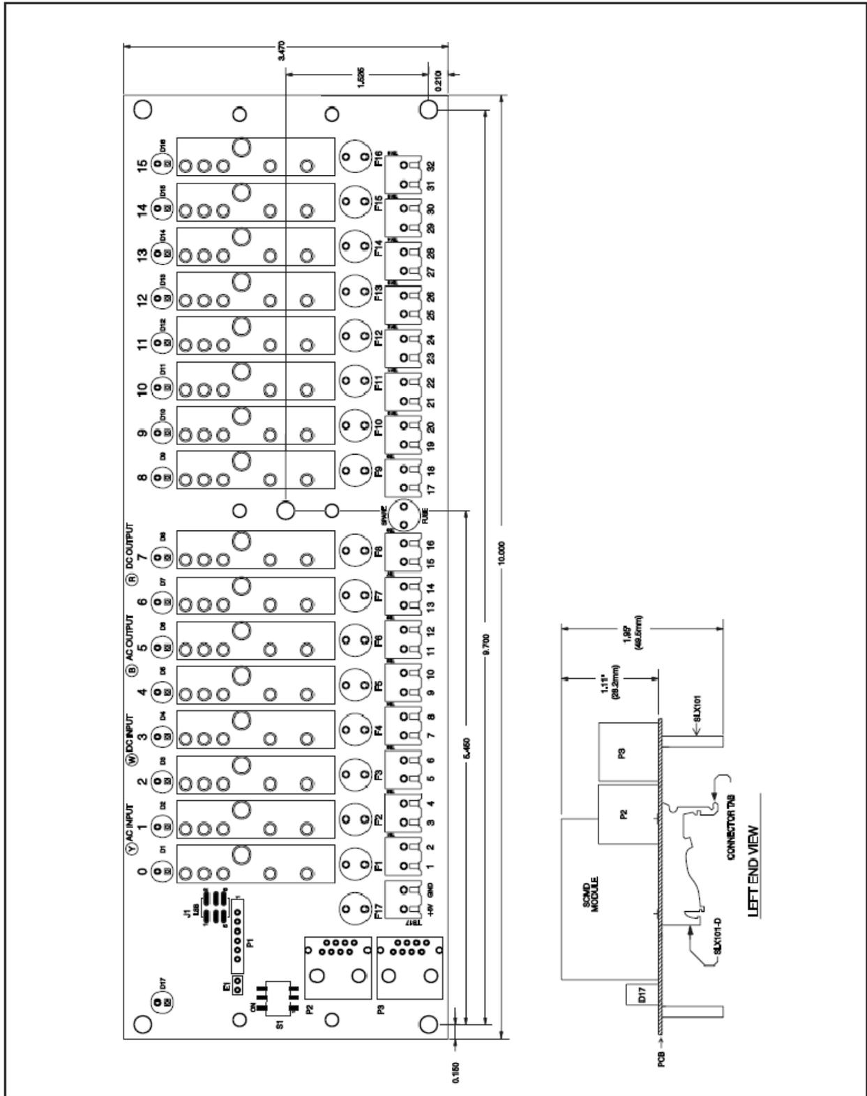
Figure 1: SCMD isoLynx® SLX101 Backpanel Dimensions
