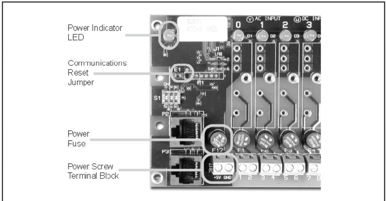
Figure 5: Digital I/O Backpanel Power Supply, Connector, and LED
