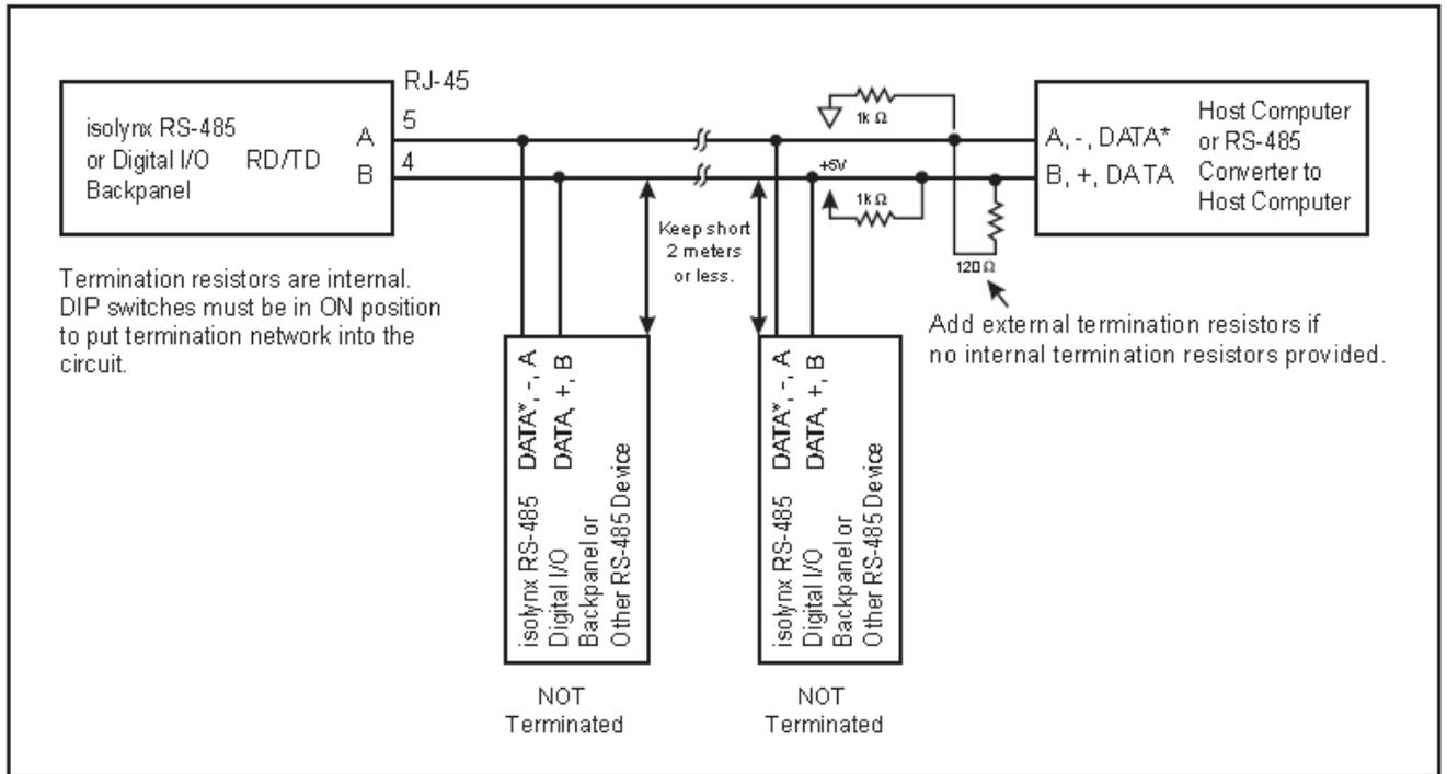
Figure B-2: Digital I/O Expansion Network Connections, Half Duplex – 2-wire, Multidrop
