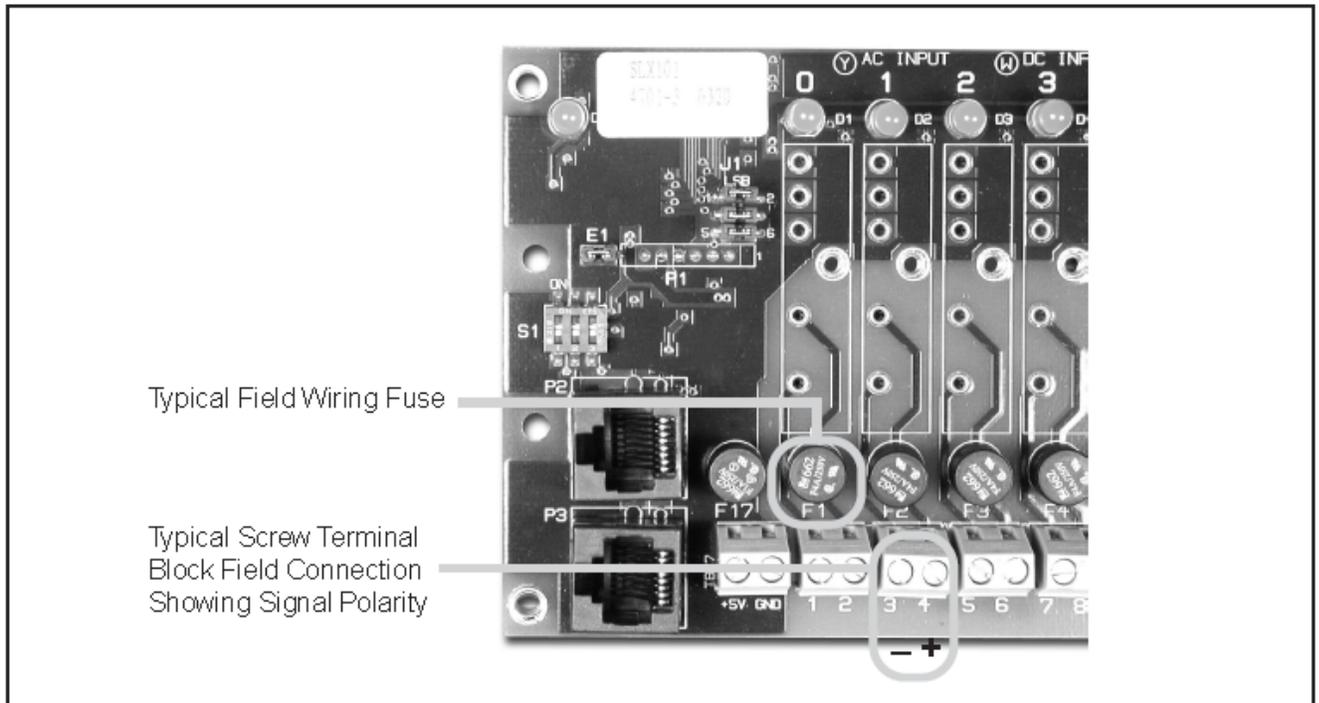
Figure 3: Signal Polarity of Field Connections
