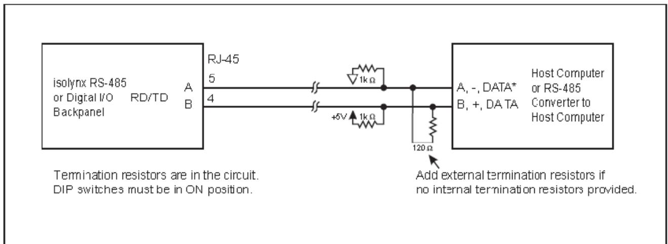
Figure B-1: Digital I/O Expansion Network Connections, Half Duplex – 2-wire, Point-to-Point
