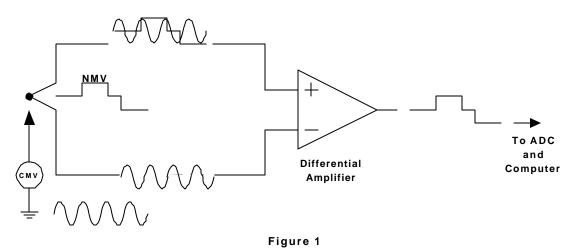
How can the comparatively expensive data acquisition instrument be used to collect the same measurements that are made so effortlessly and safely with the hand-held DVM? The answer is to choose a product that provides isolation.
