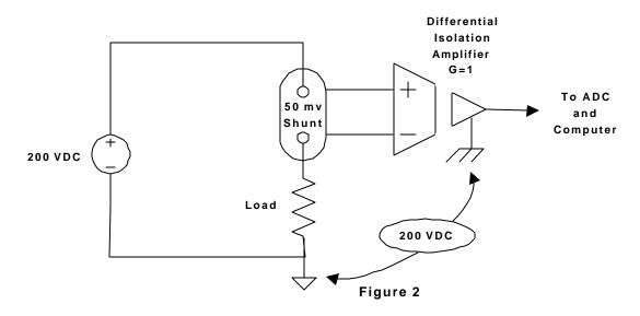
For example, with most Dataforth isolated signal-conditioning products, isolation barrier breakdown occurs above 1500V AC or 2200 VDC which is much higher than the expected CMV of most production applications. **Figure 2** (above) describes a typical application where isolation allows a measurement in the presence of a high CMV.
