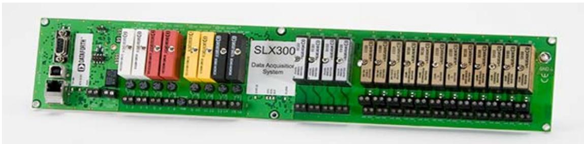
**8B isoLynx<sup>®</sup> SLX300 Data Acquisition System Hardware User Manual
